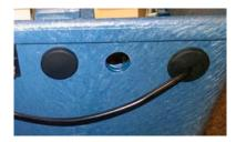
Push the connector through the mounting bracket in the inlet chamber. Please keep in mind that the level switch must be rotated 180 degrees in regards to the gravity position! Then put the nut over the connector and screw it on the level switch.
