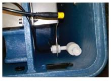
Push the connector through the opening and push it through the rubber plug. The small hole of the plug can be widened with a sharp knife to make this a little easier. Put the plug in the middle opening.
