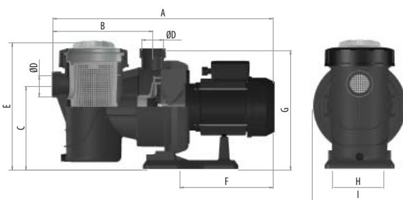
The body of the pump is made of the **latest generation thermoplastics**. The pumps are **self-priming and range from 3/4 Hp up to 3 Hp**, and are provided with both single-phase and three-phase motors. A pre-filter has been integrated into the body of the pump to prevent the entry of any foreign bodies which could cause damage to the hydraulic parts of the pump.
